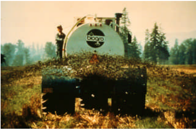
FIGURE 2 LIQUID APPLICATION OF BIOSOLIDS
