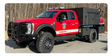
**New Forestry Truck** - This week we received delivery of our new Forestry truck. This truck replaces Engine 5 which is a 2007 and at end of life. The new vehicle was built to fight forest fires which often can be in areas that are inaccessible to our larger apparatus. It is built on a Ford F-450 cab/chassis that was upfitted with a lift kit and super single tires, carries 200 gallons of water with a 315 GPM pump and has some compartments to carry hose and hand tools.
