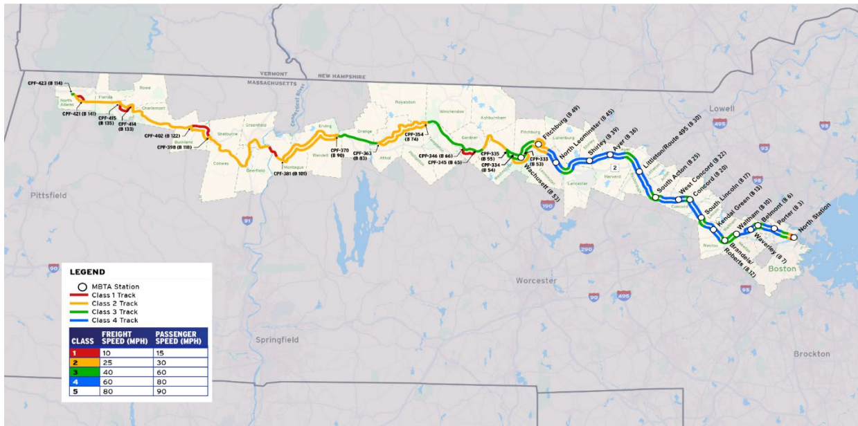
Figure 3.5: Track Classes and Maximum Allowable Operating Speeds
